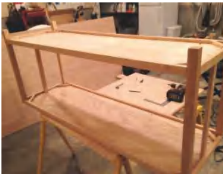
STEP 7. You then need to repeat the process for the bottom shelf with a 50mm gap for clearance under the stand. The bottom is held up by support pieces, as shown in the photo, as the corners are screwed in
